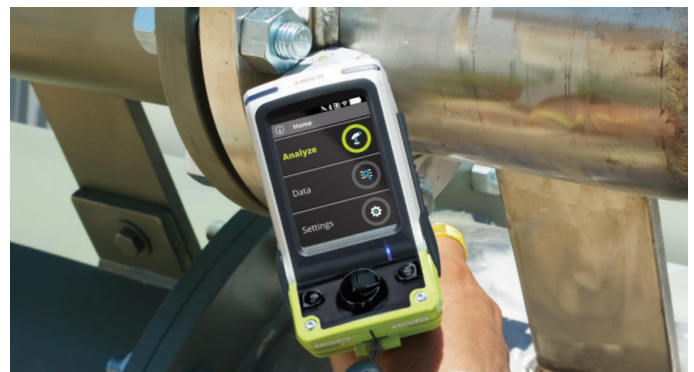
The Niton XL5 in use, analyzing a tight weld in an oil refinery.
