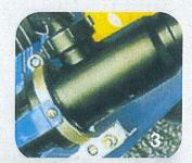
**FAN** - Cast aluminum, large diameter, aviation type centrifugal turbine. Revolution speed of 3400 RPM at 540 RPM on the tractor PTO. It can be disengaged for filling and mixing. Air speed at nozzles:
