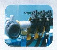
**SPRAY CONTOLS** - Manual levers with a valve for each nozzle (electric valves optional). Flow rate is controlled through an easy-to-use numbered disk. (1-10) *Photo 1*
