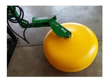
THE SPRAYDOME COVER IS DESIGNED TO GENTLY DEFLECT AND ROLL AROUND THE STEMS OF YOUNG PLANTS. UP TO 90% WATER SAVINGS WHEN YOU USE THE CDA ATOMIZER. THE SPRAYDOME 1800,2000, AND 5000 PROVIDE COVERED SPRAYING OVER 70",82", AND 196" WIDE AREA RESPECTIVELY, AND ALL CAN BE TOWED EASILY BEHIND A 4-WHEEL ATV OR WITH A THREE-POINT HITCH
