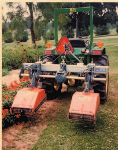
Model FP 66" frame with 2x12-16" tillage heads
