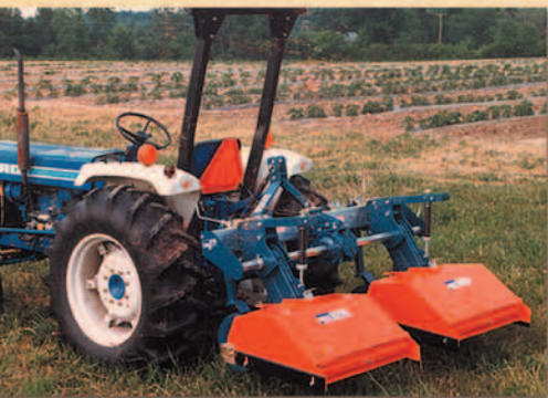
Model FL with 2 heads, clearing row middles during strawberry renovation
