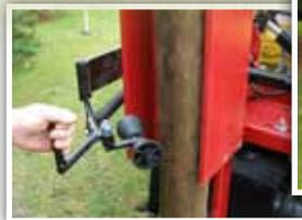
*A patented safety arm attachment holds the post in position, providing added safety for the operator.*
