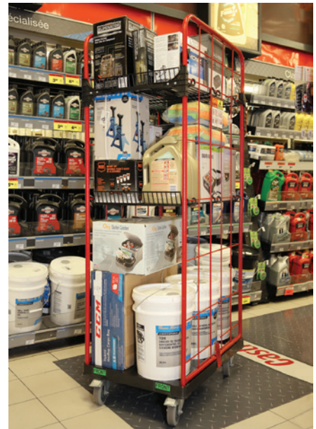
Two-shelf version used in a hardware store to move products of different sizes and to fill the store shelves on a daily basis.
