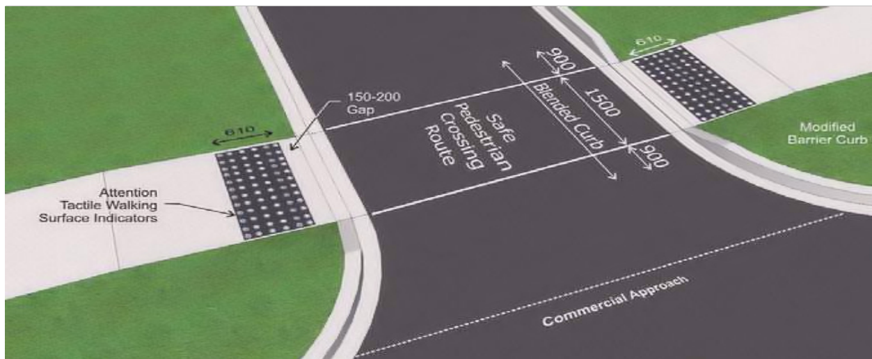
A good example of curb ramps that are aligned on the same axis.
