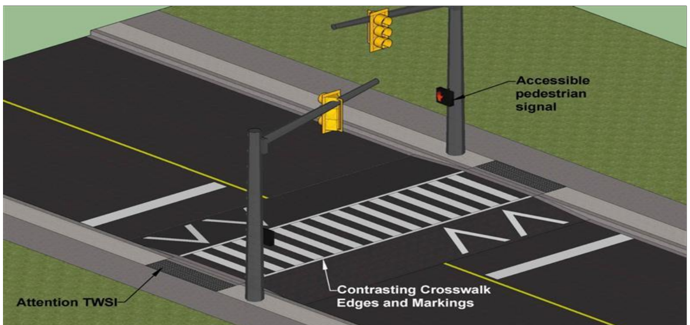
Raised pedestrian crossing at a mid-block crossing.
