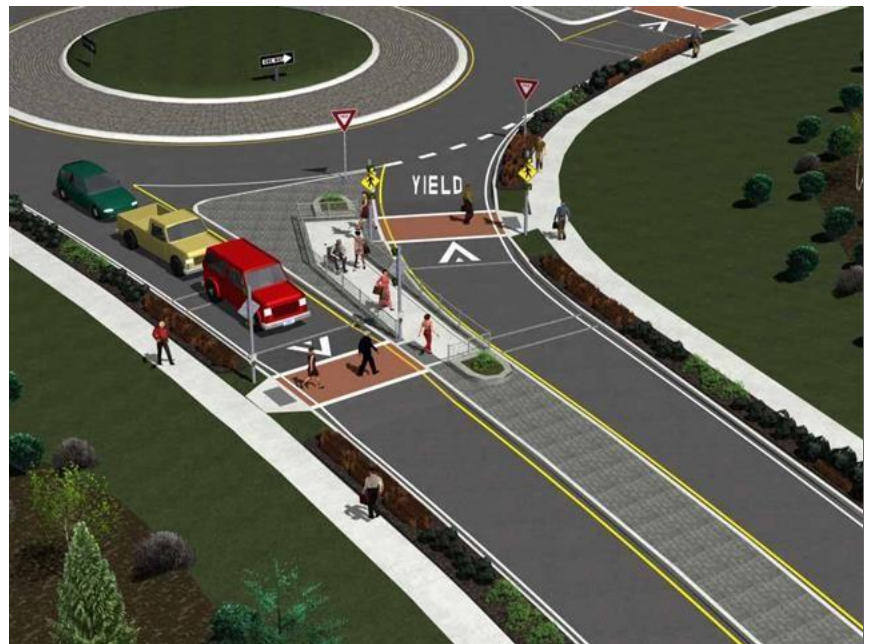
A pedestrian crossing system at a roundabout featuring an offset island in the middle of the approach road. The pedestrian route consists of a raised crossing for traffic calming. Source: Institute for Transportation Research
