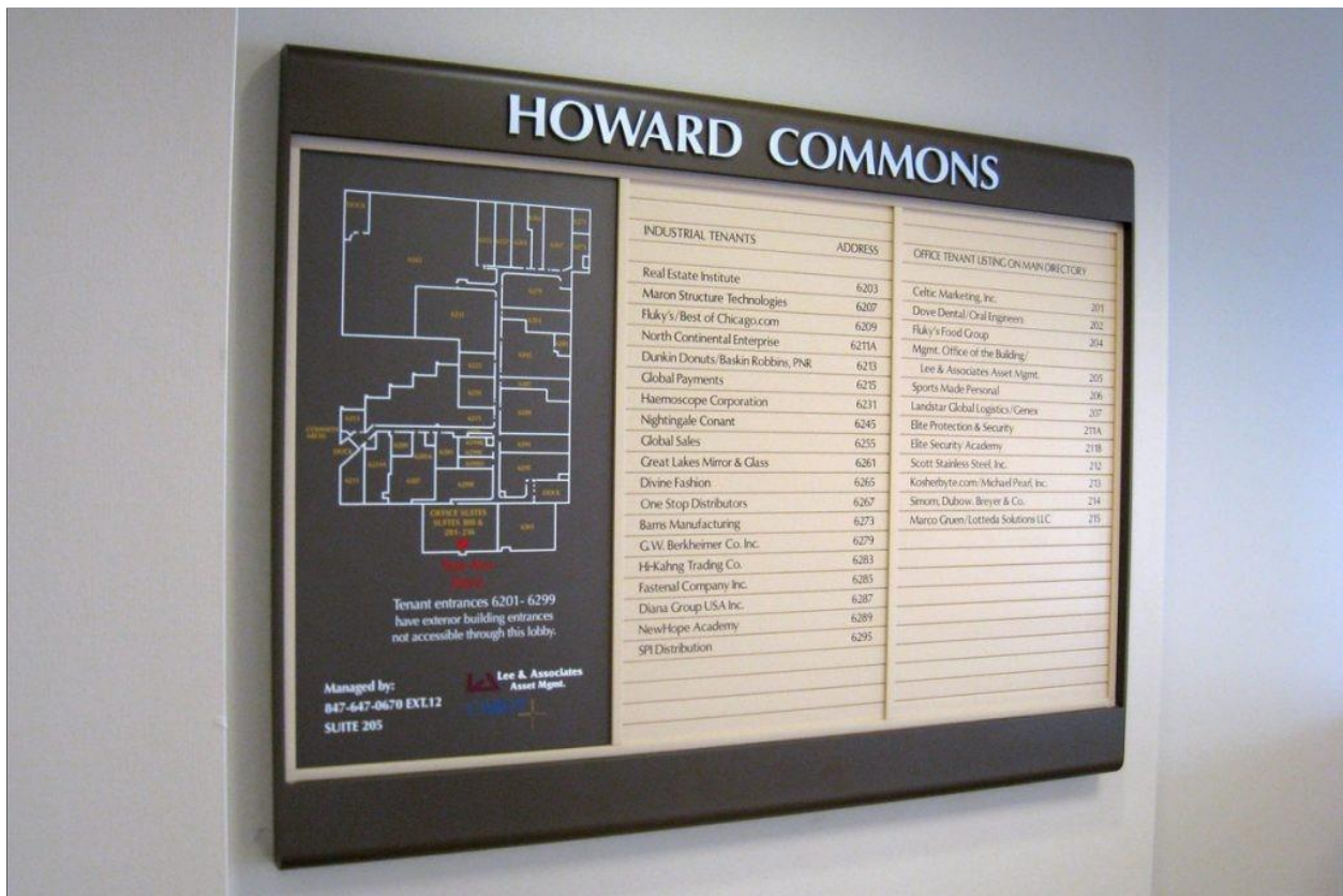
Photo example of a directory that illustrates the layout of the floor by a tactile map. Services are provided in tactile lettering.
