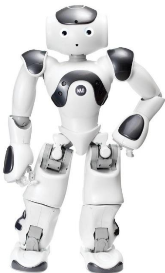
Figure 34. NAO, on the left, is a full-body humanoid robot that interacts using vocal utterances and body gestures. In contrast, Furhat, on the right, is a tabletop robot with a human-like face features.
