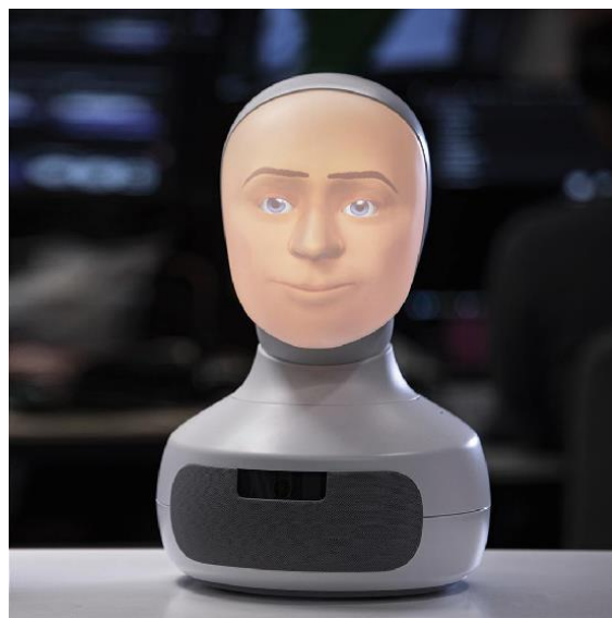
Figure 34. NAO, on the left, is a full-body humanoid robot that interacts using vocal utterances and body gestures. In contrast, Furhat, on the right, is a tabletop robot with a human-like face features.
